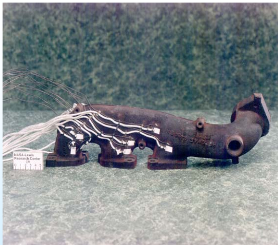
1991 R&D 100 Award PdCr wire strain gauge applied on Ford Motor Co. exhaust manifold
