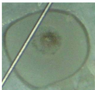
Example Failure Mechanism: Diffusion Hole Breakdown
