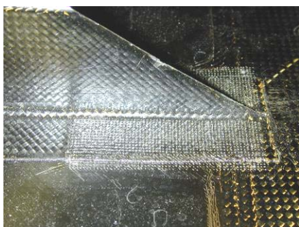
Z-pin reinforced composite flange
