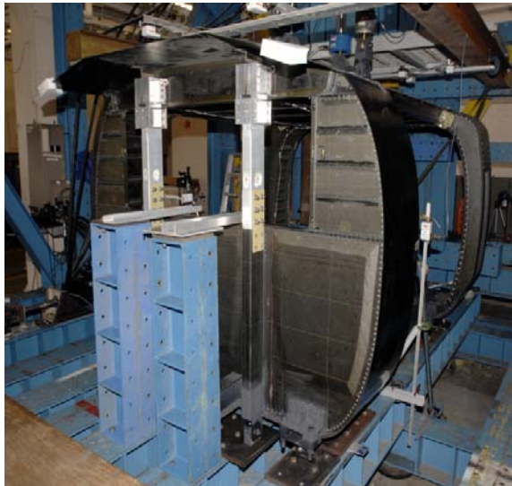
Composite fuselage section shown in the load test machine at AATD.
