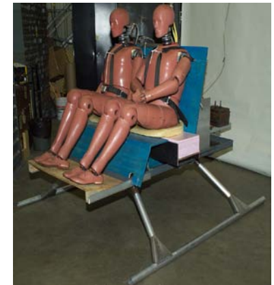
LS-DYNA shell skid gear analysis model and test article.
