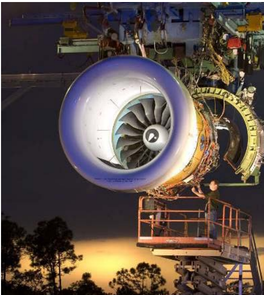
P&W GTF Demonstrator Engine Ground Test ('08)
