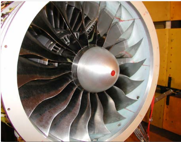
P&W GTF Model Scale Fan in 9'x15' Acoustic Wind Tunnel ('06)
