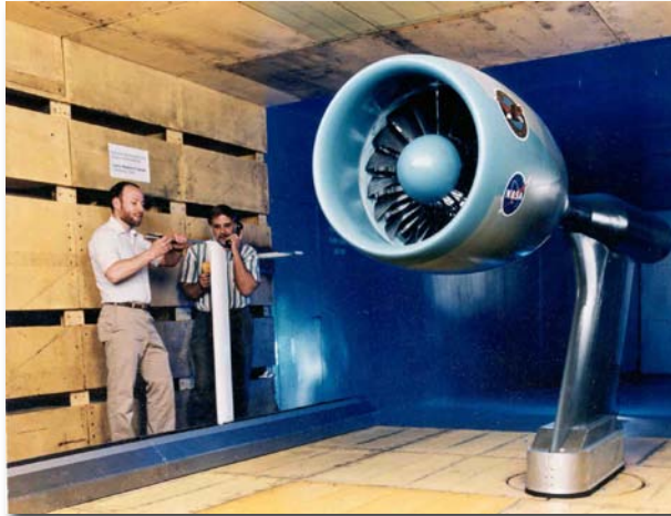
Fan Noise Reduction Technology Test-bed in 9'x15' Acoustic Wind Tunnel ('08)
