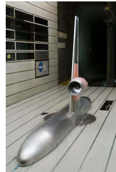
Powered Half-Span Model in 11' Transonic Wind Tunnel ('08)
