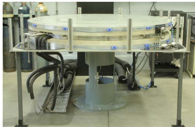
Full-scale non-actuated LIDS seal test rig
