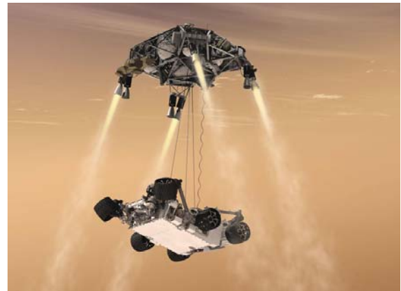
Figure 6: The Sky Crane Lowers Curiosity to the Martian Surface While Hovering with Rocket Engines.
