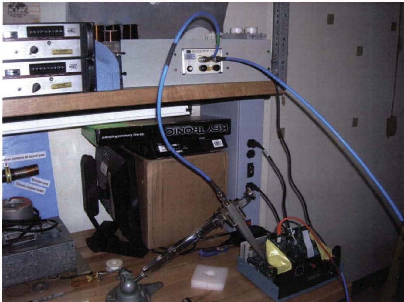
Test setup; pre-amplifier is shown at the top; near-field probe and interrogator are at lower right
