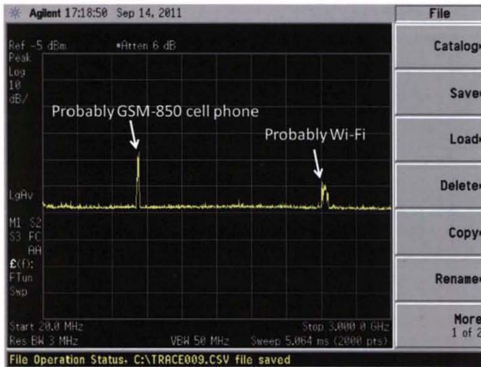
Figure 9. Spectrum of quiet EMI chamber to 3 GHz (raw data) 3
