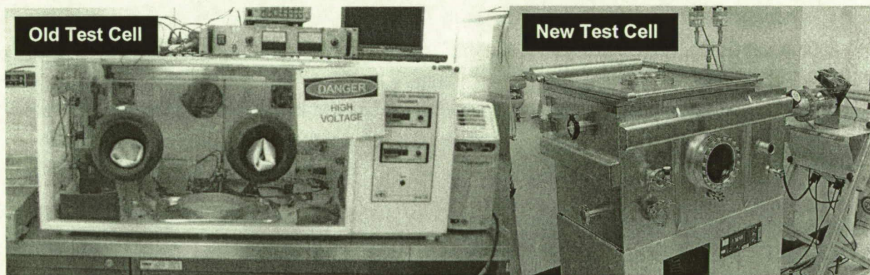
Figure 3. (Left) The ETS environmental chamber used to house the Old Test Cell for electrostatic studies of MLS-1 under dry ambient conditions. (Right) The high vacuum chamber used to house the New Test Cells for testing under simulated lunar environmental conditions.
