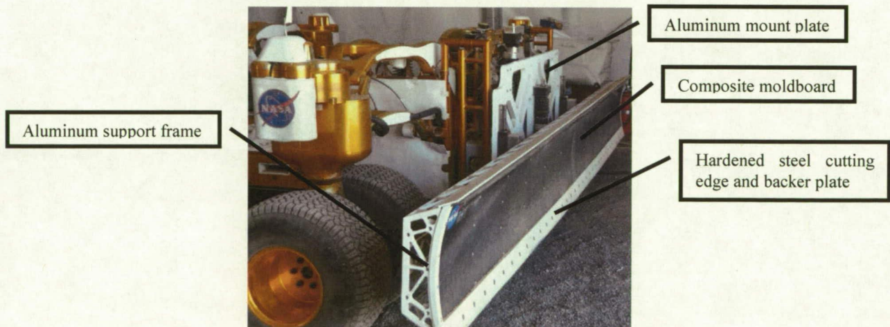
Figure 6: Lance blade diagram mounted on Chariot
