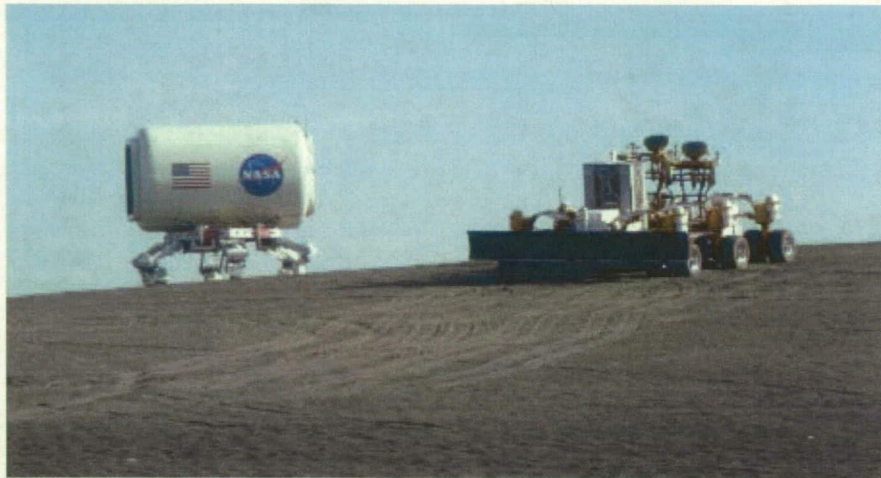
Figure 12 - LANCE blade attached to Chariot (right) and ATHLETE with habitat (left)
