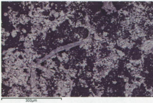
Figure 5. QBSD of NVR debris solids.
