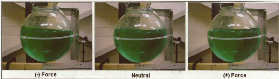
Figure 9: Natural damping slosh positions for 60% fill level
