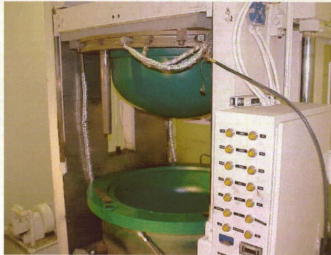
Figure 17: Elastomeric rubber fabrication and diaphragm molding (Courtesy: PSI)
