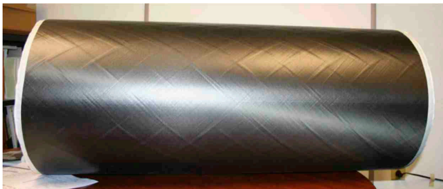
Figure 2. Advanced composite tow-steered shell
