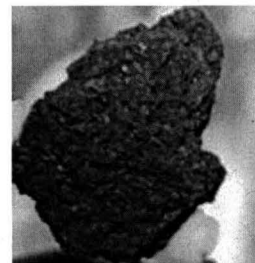
Figure 1. Biochar's high carbon content and porous nature can help soil, and possibly regolith, retain water, nutrients and microbes. Source CNN.
