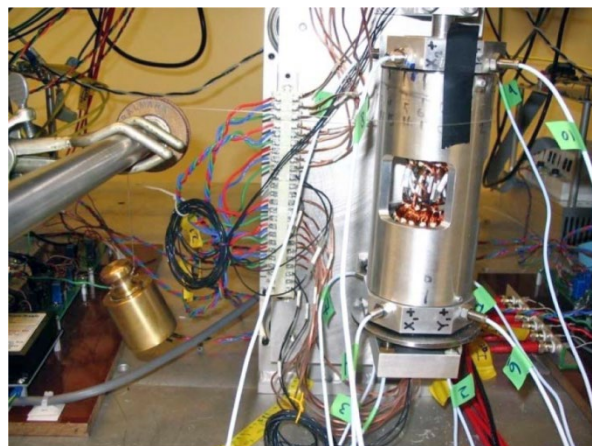
Figure 16.—Force applied to bearingless machine.
