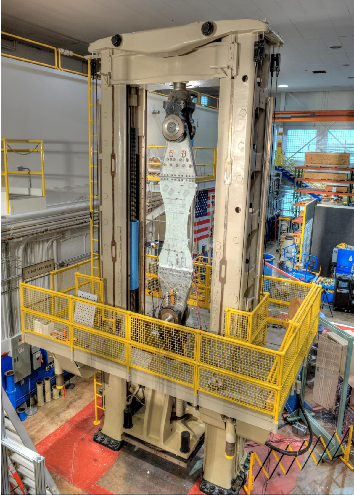
Figure 7. Repaired tension PRSEUS panel installed in the one million pound test machine at NASA LaRC.
