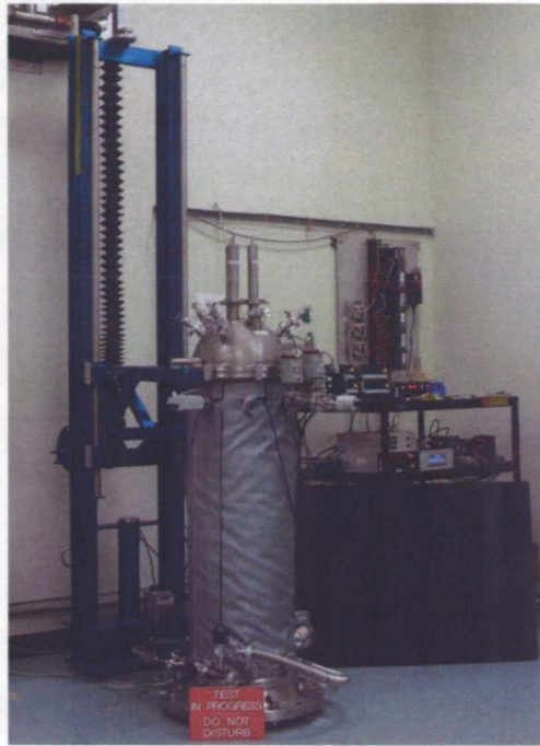
FIGURE 1. Overall view of the Cryostat-100 test apparatus and system for determining the absolute k-value for a cryogenic thermal insulation system.
