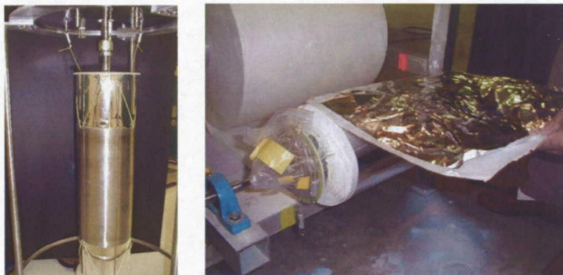
FIGURE 1. Cryostat-2 cold mass shown before (left) and after (right) roll-wrapping with insulation materials.
