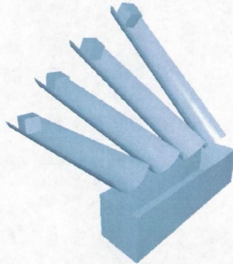
Figure 5. EDEM Model of four inclined curved surfaces at 0°, 15°, 30°, and 45°. Box structures on the end are the particle factories.
