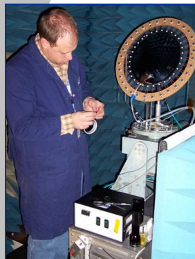
0.3 meter prototype Membrane reflector
