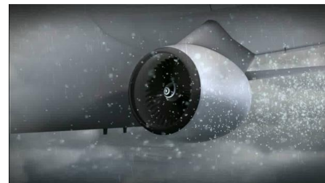
Artist rendition of the engine icing accumulation and shedding.
