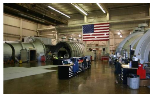
NASA GRC Propulsion System Laboratory to be modified to run engine icing conditions.
