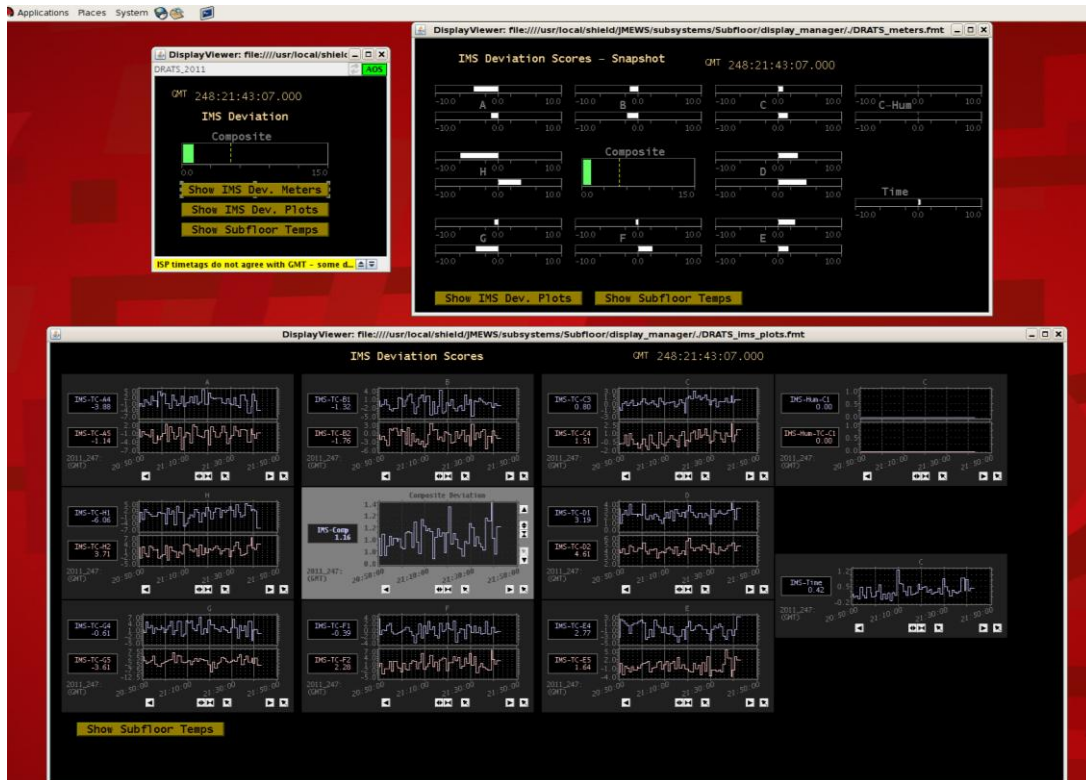
Figure 2: Anomaly detection display formats. Upper left display shows a meter for the instantaneous value of the composite deviation score. Upper right display shows meters for the instantaneous values of each of the parameters being monitored. The meters are arranged to parallel the clockwise arrangement of HDU segments A through H with two temperatures per segment. We also added a time-of-day parameter to accommodate possibly different behavior during day and night operations. The bottom display graphically shows deviation scores over time arranged as in the meters display.
