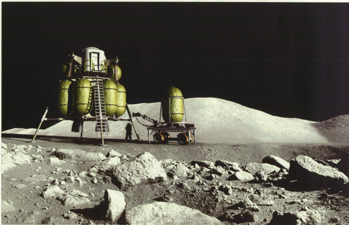
FIGURE 5. Artist conception of transfer operation of consumable liquid or vapor between LSAM and ground storage tanks.
