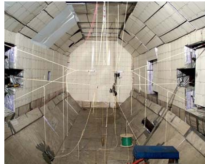
Figure 8. Inside view of the Range G target chamber. The interior of the range tank is populated with low density foam panels.
