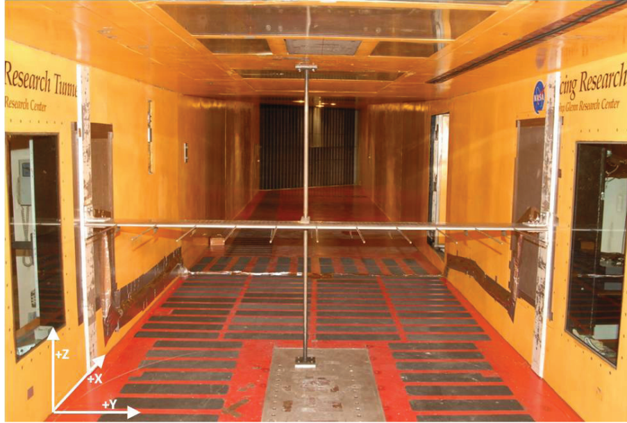
Figure 3: The 9-foot horizontal survey rake installed at vertical centerline in the IRT test section
