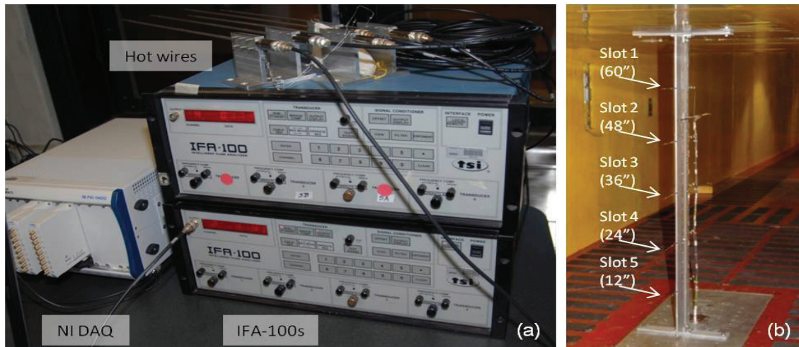
Figure 11: Hot-wire/film anemometry system: (a) NI DAQ and IFA-100 (b) hot-wire rake installed in the IRT test section with five hot-wires and a pitot-static probe
