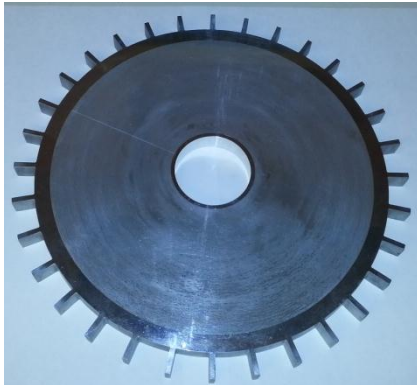
Figure 8. The 12.7-mm thick, 254-mm diameter aluminum disk that will be tested in the Rotordynamics Lab.
