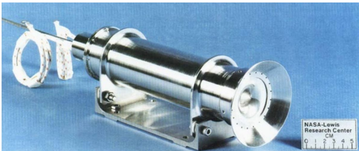
Figure 5.—Resistojet thruster engineering development model (Ref. 34).
