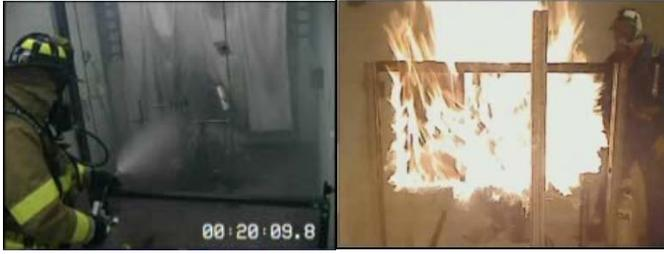
**Figure 9. EDU discharge against the stored energy battery fire (left) and prior to discharge against an open cabin fire (right).**
