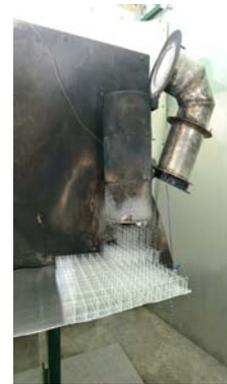
**Figure 5. ISS stored energy oxygen candle configuration.**
