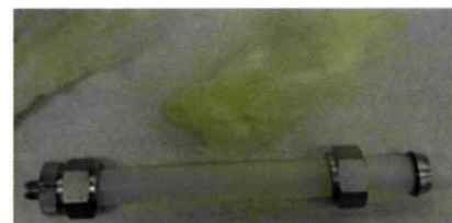
Figure 3. Glass wool, initially white, turned yellow from tar capture in the filter.
