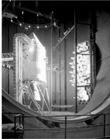
Boilerplate Apollo S/C 008 in Chamber A with side-sun solar
