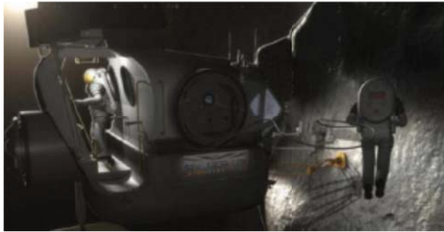
Figure 9 Simulation View of Asteroid EVA RATS 2012 utilized a simulated asteroid that was tied to a real live MMSEV and crew along with EVA crew participating in Virtual Reality and/or simulated (suspended) weightlessness.
