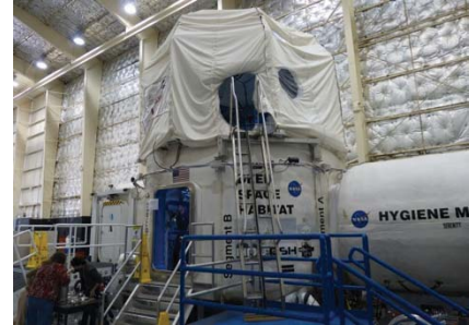
Figure 17 Deep Space Habitat prototype used in the AMO project simulation Shown with inflatable upper section provided by a university as the winners of a competition of inflatable habitat designs.
