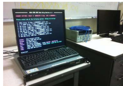
Figure 23 Communications Delay Emulator The network delay emulator allowed the analog missions to configure the communications time delay as well as the data bandwidth and link quality.
