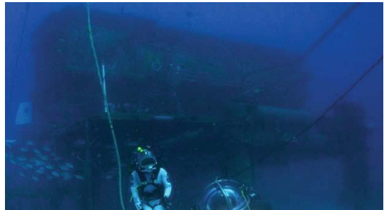
Figure 3 Human-Robotics Testing Deepworker subs carrying crewmembers on platforms to simulate EVA operations at an asteroid (Aquarius in the background).
