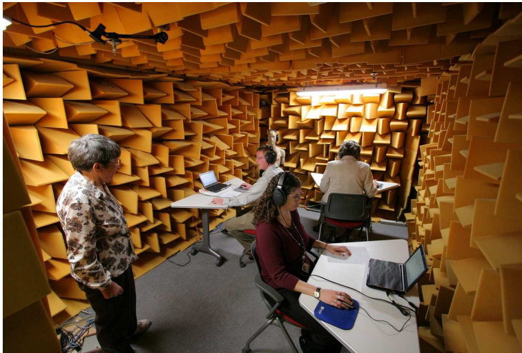
Figure 5. Headphone test setup in a small anechoic chamber at NASA Langley Research Center.
