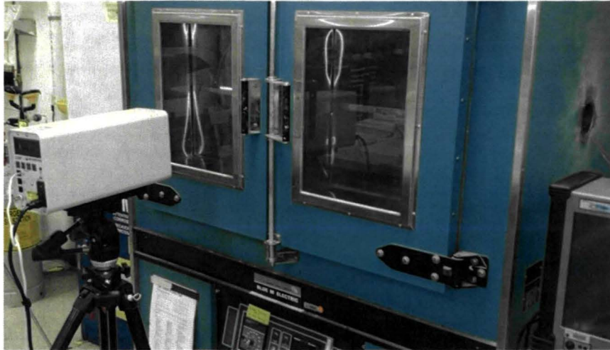
Figure 8: Test Setup with Laser Extensometer
