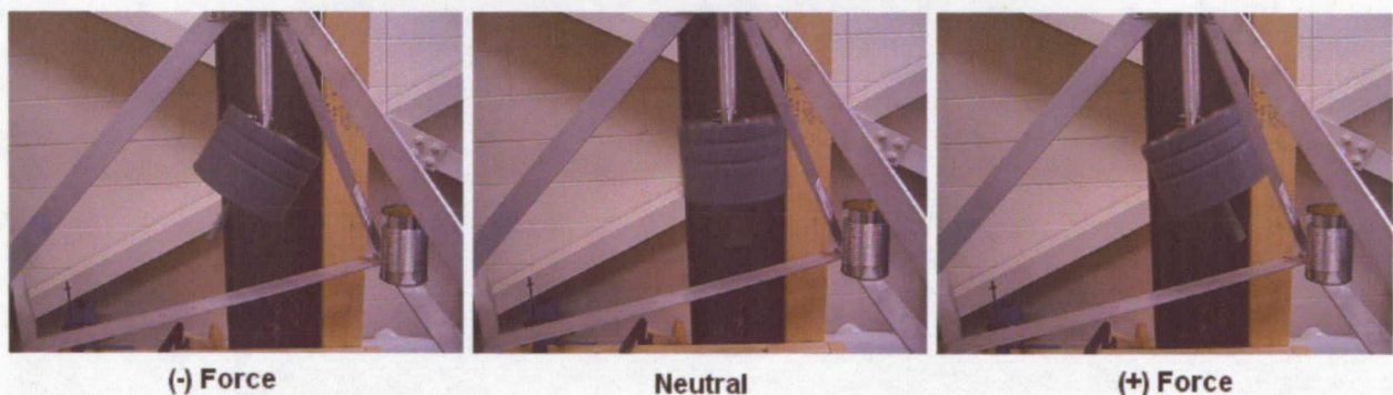
Figure 1: Mechanical analog of lateral free-surface fuel slosh.
