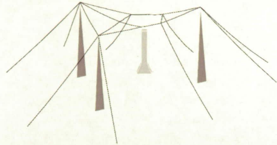
Figure 7. Isometric view of the lightning protection system of LC39B at the Kennedy Space Center.
