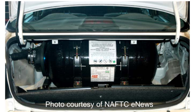
Composite Pressure Vessel “Green” Fuel Container Installation
