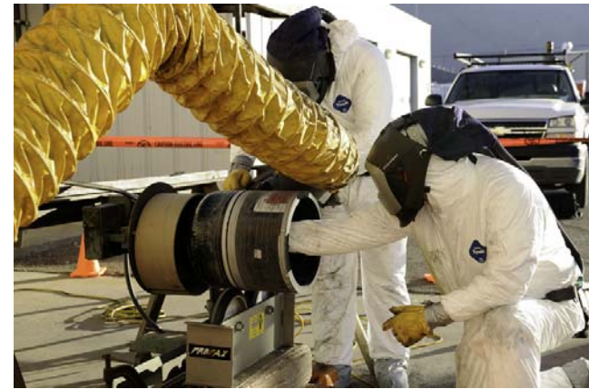
NASA White Sands Test Facility Personnel Cross-sectioning a CPV Fuel Container
