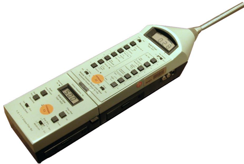
Figure 4. Brüel & Kjær Type 2231 Modular Precision Sound Level Meter with the Type 1625 One-Third Octave Filter Set and the Type BZ7108 Reverberation Processor.
