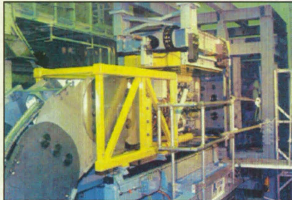
Atlas V Autocoupler Assembly At KSC Test Site
