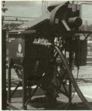
FIGURE 4. The portable dust collection system designed for offloading bubbles in remote locations.
