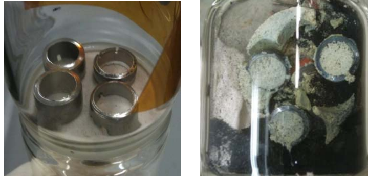
FIGURE 4. Material candidate samples in the sublimator before and after CVD operation.
