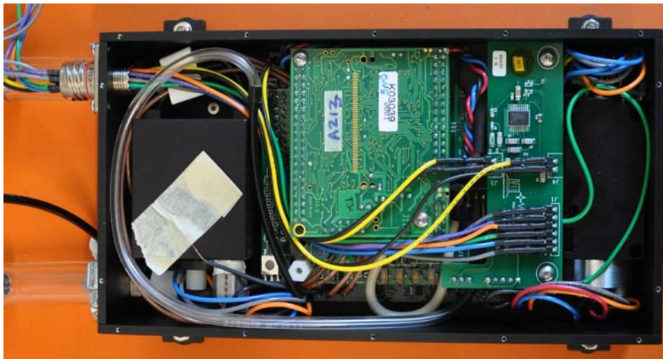
Figure 13. Integrated Version 2.0 sensor. Optical and electronic layout after full conversion to 2.0 architecture. An RS-485 bi-directional interface and power supply board compatible with the APLSS 2.0 system has been added.
