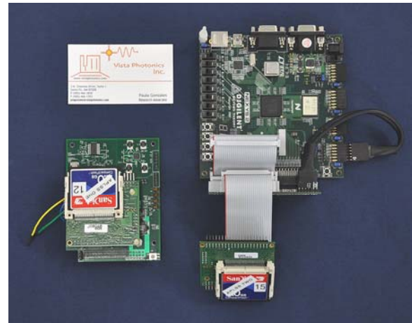
Figure 4. Custom and COTS FPGA. Reduction of the electronics footprint was enabled by using the custom FPGA board in the left of the photograph.
