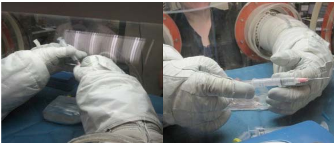
Figure 16. Gloved assessment of syringes. Different syringes were manipulated with EVA gloves in a simulated pressure environment to determine how the geometry and size of a potential injection device affects a gloved operator’s ability to provide an injection.
