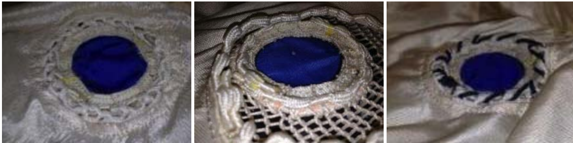
Figure 4. Various David Clark A-1C injection patches. Left to right: Injection patches from A-1C serial numbers 114, 133, and 125.
