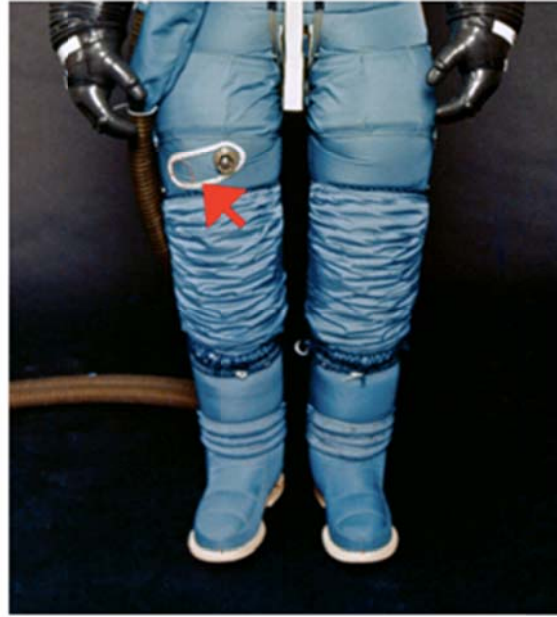
Figure 7. A7L LCG (left) and suit with TMG removed (right). The LCG tubing of the A7L suit was strategically routed to avoid needle puncture if the injection patch was used.
