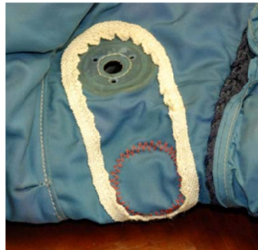
Figure 6. Injection Patch from A7L SN 053. Injection patch from Frank Borman's A7L suit as viewed with the TMG removed.
