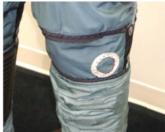
Figure 8. A7L/B injection patch. The patch was relocated from the right to the left thigh for the A7L/B.
