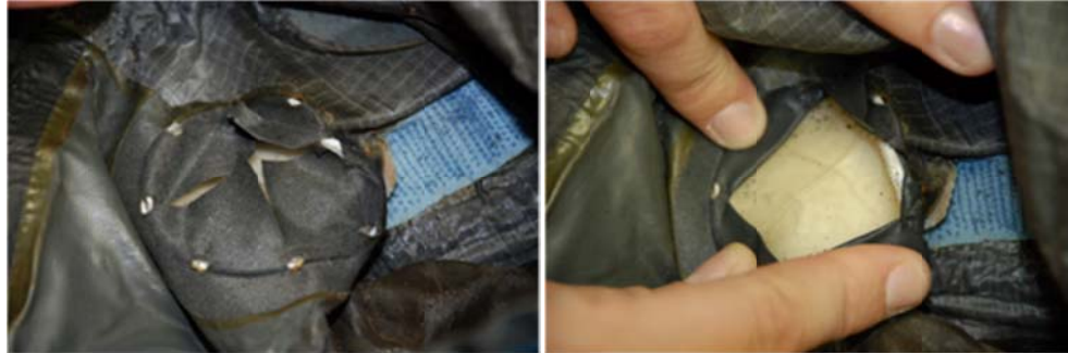
Figure 10. Removal of injection patch from A7L suit. An incision was made from inside the bladder, as shown on the left. The injection patch can be clearly seen in the photo on the right.
