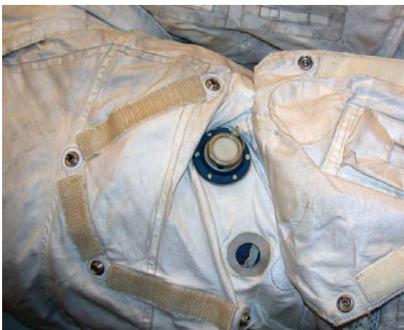
Figure 9. Ed Mitchell's A7L suit from Apollo 14. Shown is injection flap, UTC, and edge of injection patch.
