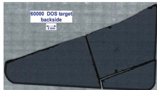
Figure 4: This photo shows the target wafer after cleaving scribe lines 1 & 2. The requested allocation piece is in the upper right hand section of the photo.
