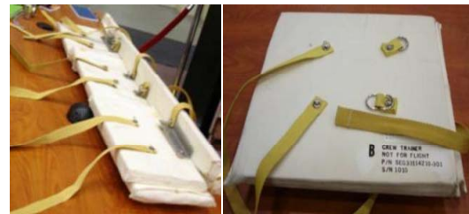
Figure 10. TeSS brick assemblies – custom and flat bricks.
