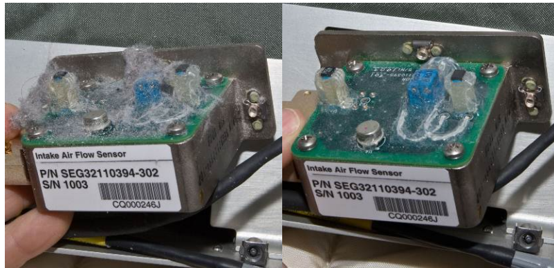
Figure 2. Starboard CQ intake air flow sensor (pre and post cleaning).
