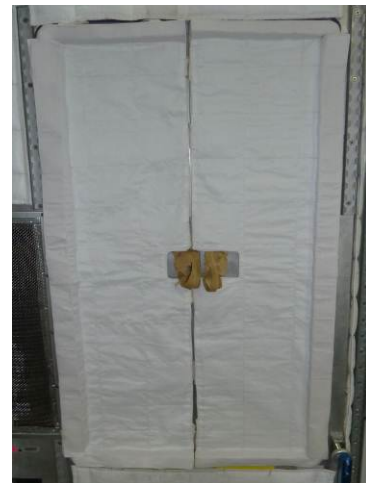
Figure 8. Cover installed on CQ exterior doors.
