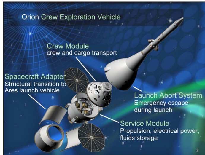
Figure 1.—Schematic of the Orion Crew Module and supporting systems. The fairings can be seen as the three semi-circular shells in the exploded view of the spacecraft adaptor. (Figure from NASA: JSC2009-E-145322)
