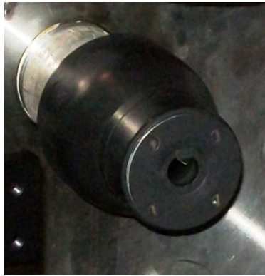
Fig. 7 The convergent nozzle with a single delta-tab installed in the free jet facility.
