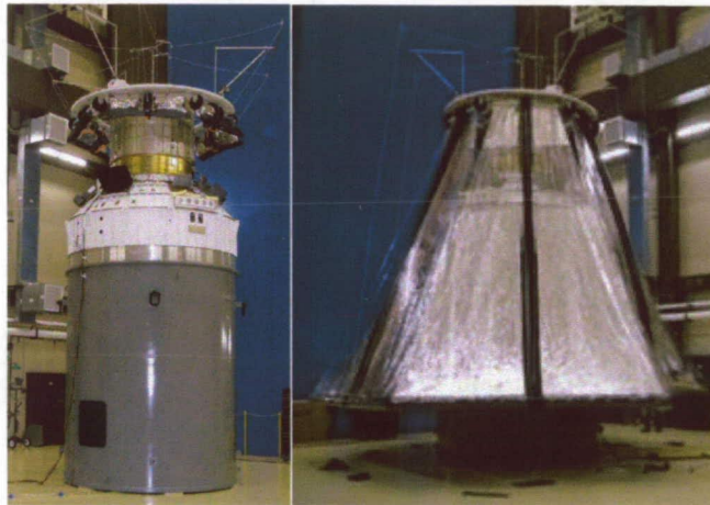
Figure 2: CSS 2007 Deployment Test; Stowed & Deployed Configurations
