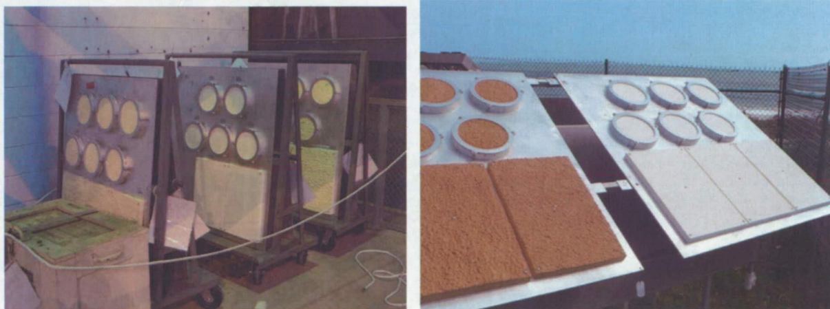
Figure 4. Exposure testing of SOFI test specimens at the Kennedy Space Center. Aging inside the Vehicle Assembly Building (left) and weathering at the Corrosion Beach Site (right).
