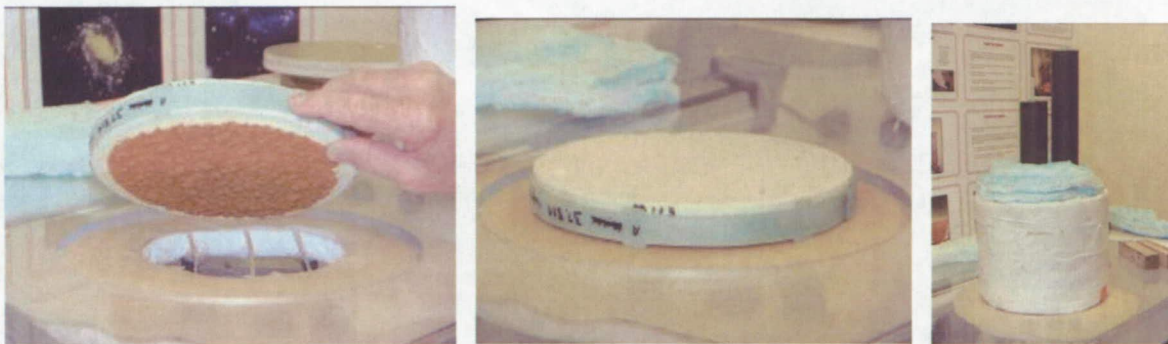
Figure 2. Installation of SOFI test specimen is shown in the photographic sequence from left to right. The weathered side (dark orange color) is placed downward into the environmental chamber while the non-weathered side (light yellow color) is facing the cold mass assembly on top.
