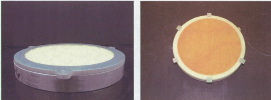
Figure 3. The foam specimen mounting enclosure (left) was designed to expose only the center portion of the top face of the material. The photo on the right shows BX-265 after only one month of weathering.
