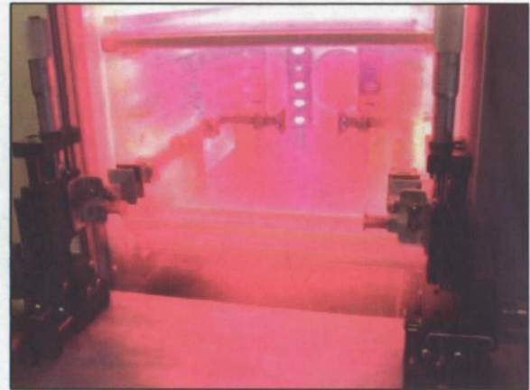
Figure 1 Studying millimeter wavelength signal attenuation through plasma at Kennedy Space Center inside a plasma chamber
