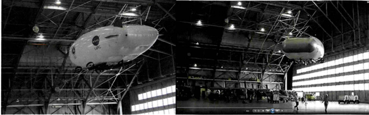
FIGURE 44: VIDEO SCENE OF THE INDOOR FLIGHT TEST OF THE SOLAR AIRSHIP
