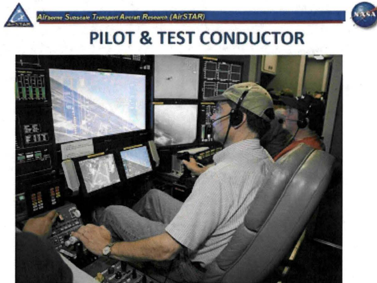
FIGURE 37: AIRSTAR REMOTE INTERNAL PILOT AND GLASS COCKPIT CONFIGURATION LOCATED INSIDE THE MOS
