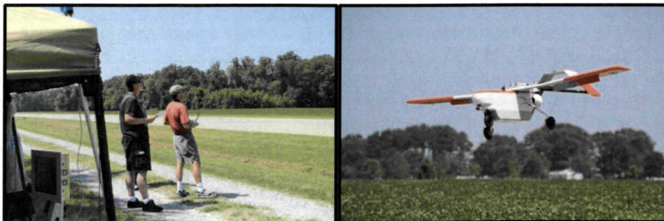
FIGURE 36: AIRSTAR BAT-4 EXPERIMENTAL TEST-BED BEING FLOWN BY AN EXTERNAL PILOT IN RC MODE WITHIN VISUAL LINE OF SIGHT
