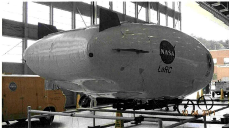
FIGURE 45: FULLY ASSEMBLED SOLAR AIRSHIP WAITING FOR FLIGHT TEST SECURED TO TIE DOWN STRUCTURE
