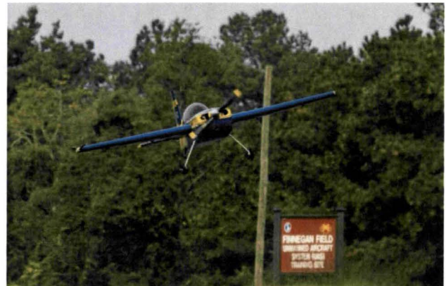
FIGURE 46: EDGE 540T 33% SUBSCALE VEHICLE BEING FLOWN AT FINNEGAN FIELD, FT. A. P. HILL, VIRGINIA
