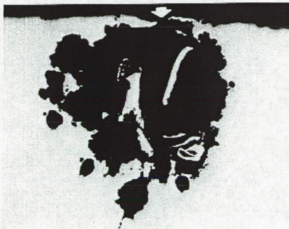
FIGURE 1. Micrograph (100x magnification) of pit from KSC's launch pad S30403 SS tubing.
