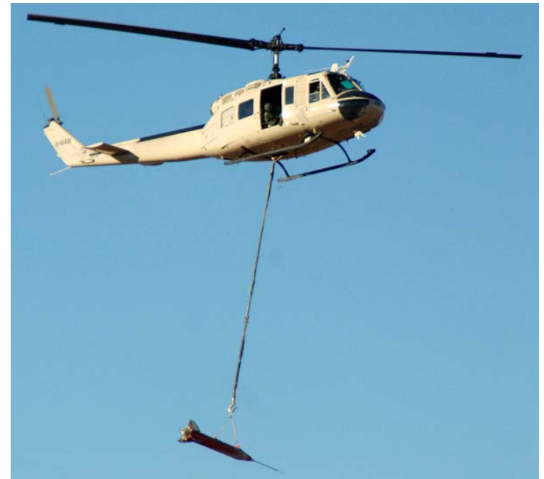
Small DTV Suspended Beneath UH-1
