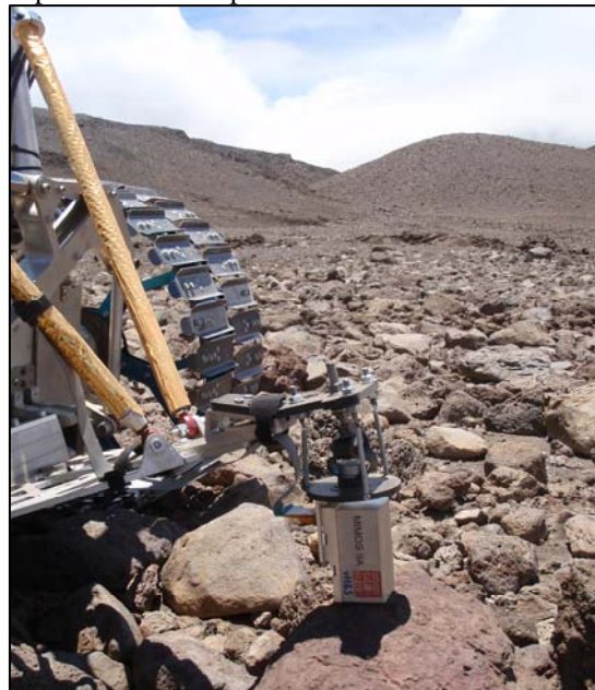
Figure 1: MIMOS IIA sensor head deployed from the JUNO II rover on a rock target in Apollo Valley.
